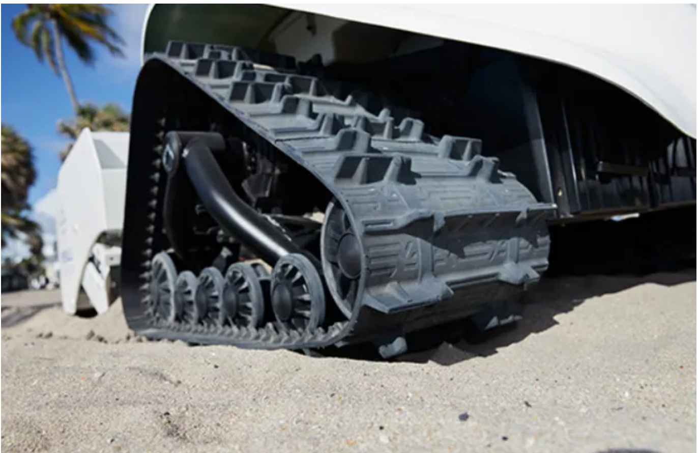
Operated remotely, the BeBot traverses sandy areas, raking for debris and leveling out beach expanses. Provided by The Tip of the Mitt Watershed Council
