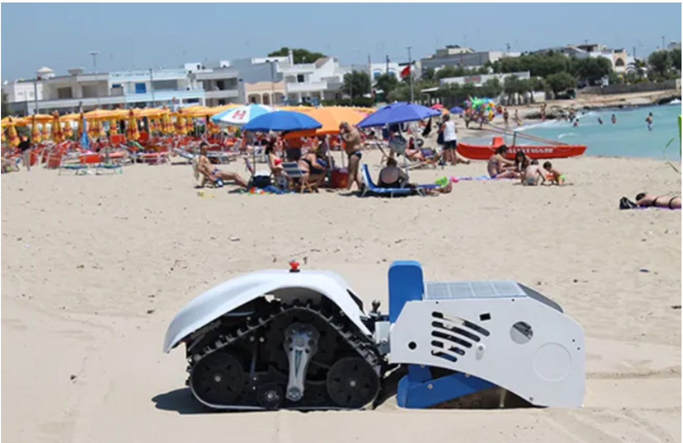
The BeBot, powered by batteries and solar energy with a three-hour maximum operational duration, is scheduled to operate twice a week from May to October on select beaches in Northern Michigan. Provided by The Tip of the Mitt Watershed Council
